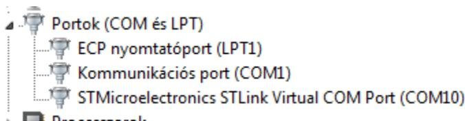
If so, your computer has recognized the driver and can communicate with the analyzer.
